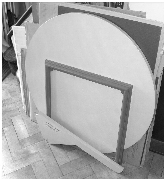
Fig. 2. Wynne & a vertical dial frame patterns for casting.
