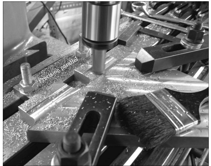
Fig. 6. Milling tenons to thickness.
