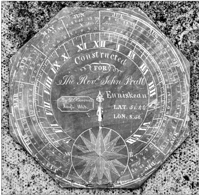
Fig. 1. The unrestored dial plate dusted with talc to bring out the detail.
