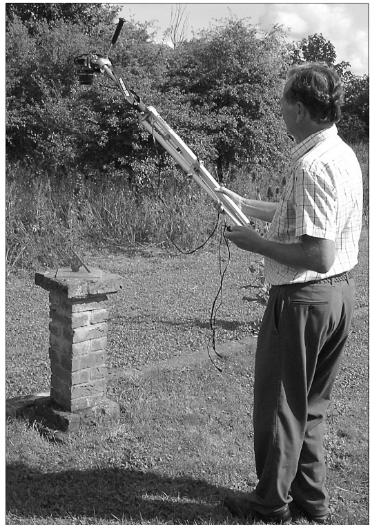
Fig. 5. 'Extended tripod' technique used for getting a good overhead shot a garden dial.
