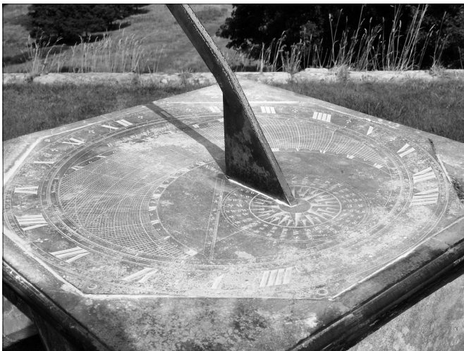
Fig. 5. The Wynne DH dial at Powis Castle, October 2005. The gnomon remains bent.....
